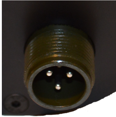
Figure 10 - MIL-C 5015 10SL3S connector of the device
