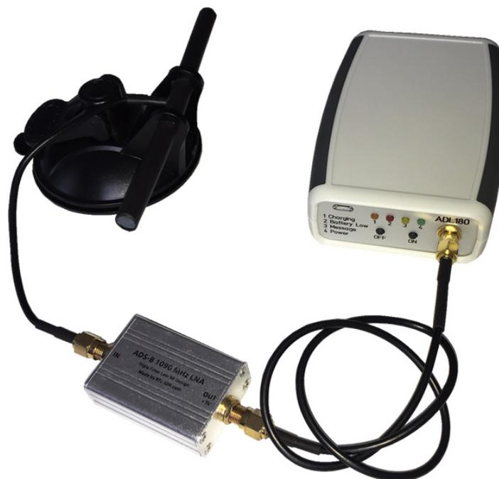
Figure 6 ADL180 with optional ADS-B amplifier and antenna
