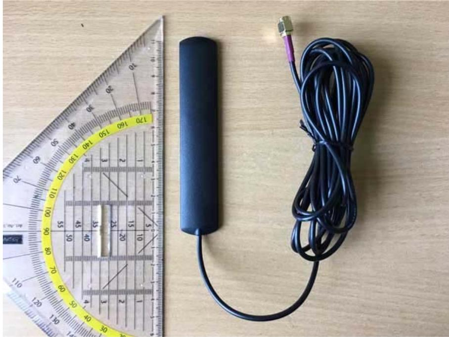
Figure 3 ADS-B Antenna
