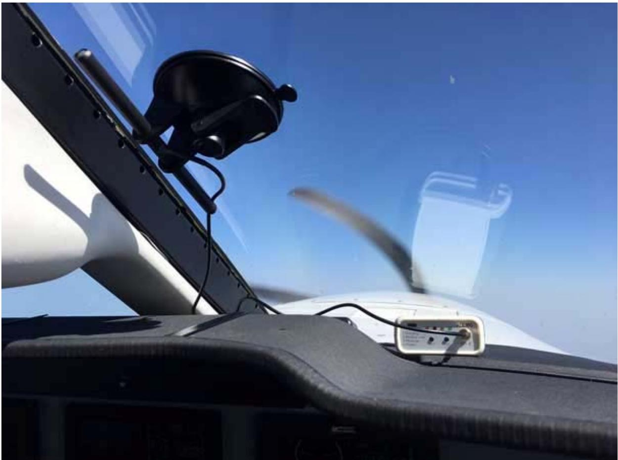
Figure 2 ADL180 on the glare shield in the right orientation with the suction cup antenna
