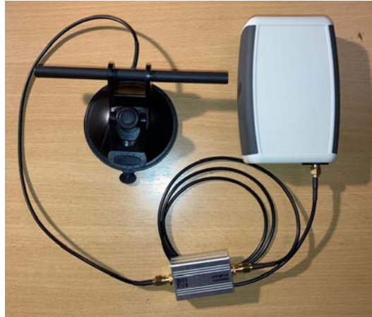
ADL180 with suction cup antenna, optional amplifier and wiring
