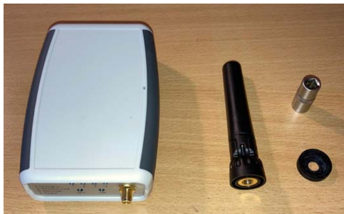
Required materials for the folding antenna installation
