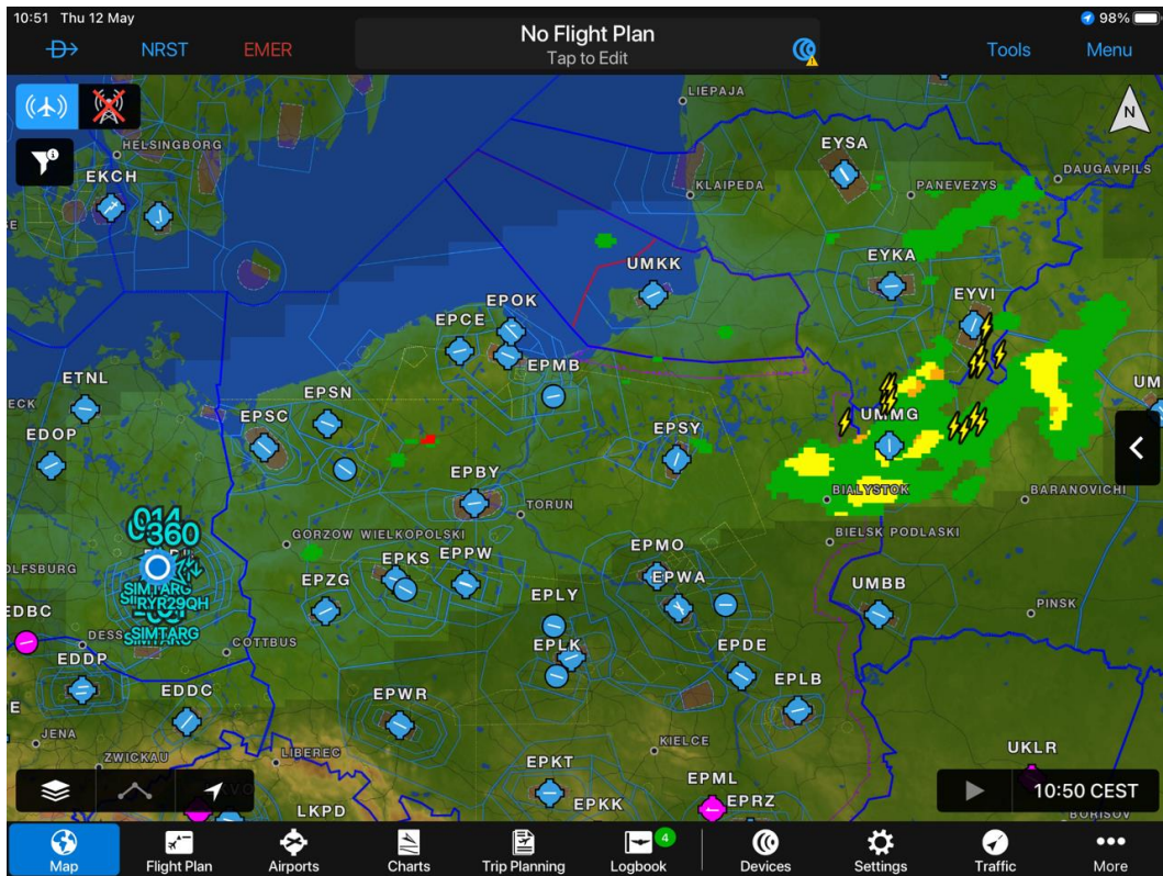
Figure 11 ADL200 weather data and stratux traffic displayed in Garmin Pilot
