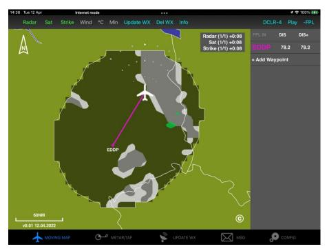
Figure 5 ADLConnect Displaying the Latest Weather Data
