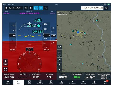
Figure 14 ForeFlight Displaying Synthetic Vision and Traffic Broadcasted by ADL200
