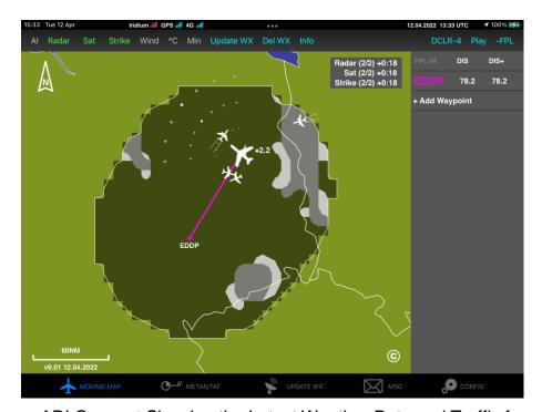
Figure 8 ADLConnect Showing the Latest Weather Data and Traffic from ADL200
